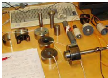
Figure 4. Gripper head shapes tested
