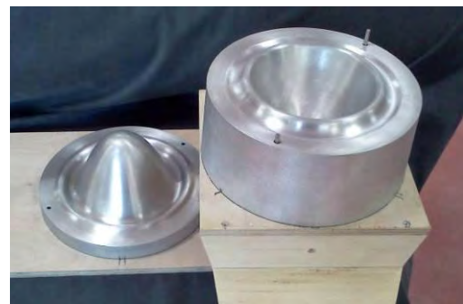
Figure 2. Reference lab-scale mould (paraboloid) for one-step thermoforming
