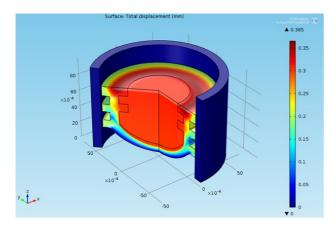
Figure 1: Computed displacement of plunger tip in contact with syringe glass barrell
