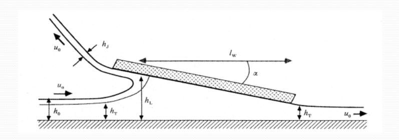
Sugimoto's schematic representation of the planning of a skim board over a thin water layer used to develop the COMSOL model.
