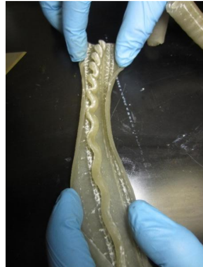
Figure 15: extrudate quality without the heat transfer effect of the mid layer material.
