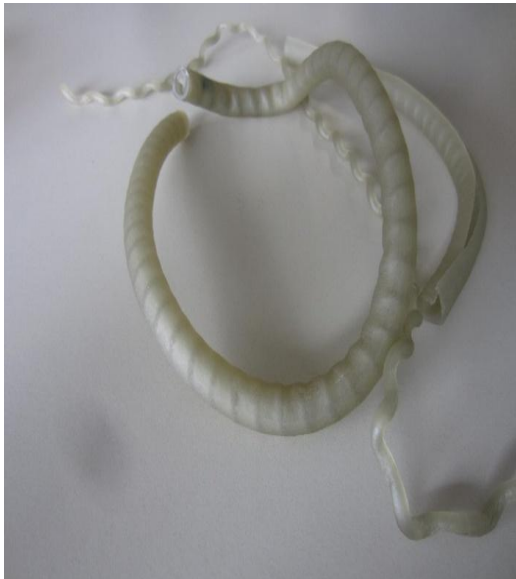
Figure 14: Extruded strand with inner section of air.
