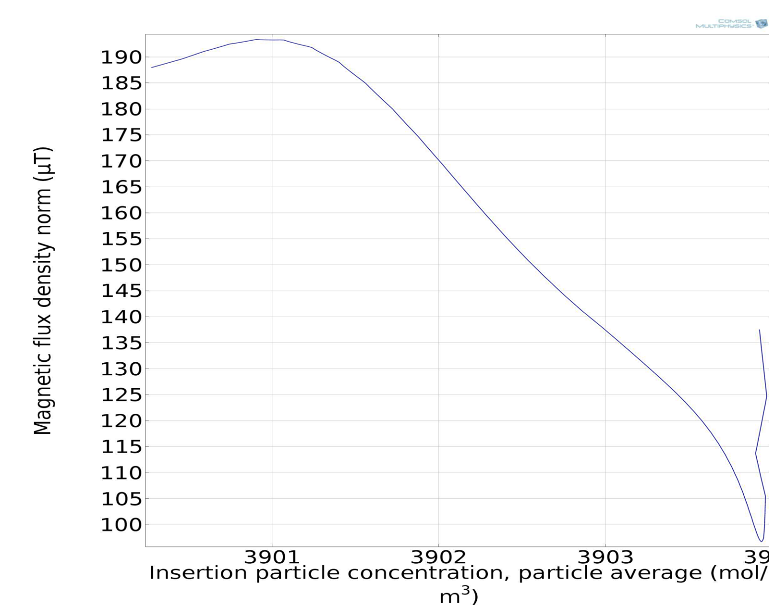
Figure 3. Insertion Li-ion particle concentration Vs. Magnetic field response
