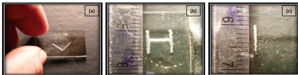
Figure 2: Different types of microchannels on glass (a) V- type (b) H- type (c) I- type.
