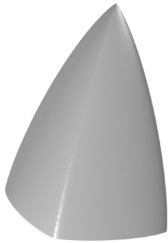
Figure 3: Morphology of a single widmanstatten ferrite plate in 3D by PFM.
