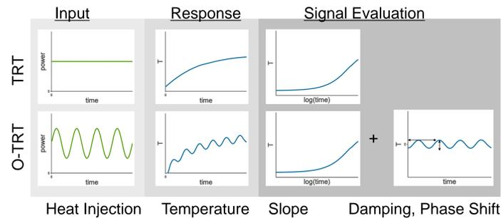
The idea is to add an oscillatory part to the constant heat injection. The system response is a superposition of constant and oscillating heating. **The constant part can be evaluated conventionally, the oscillation contains further information about thermal properties.** The amplitude and phase shift are functions of thermal conductivity and heat capacity. The **penetration depth** depends on the frequency of the signal and can thus be adjusted to expand only into certain regions.
