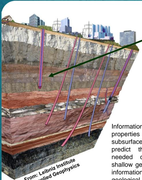
**Geothermal Energy** is a growing branch of sustainable energies. We focus on **shallow geothermal applications**. A common setup is a **Borehole Heat Exchanger (BHE)** of typical depth between 20m and 300m with a single or double u-pipe inside. The subsurface is used as thermal source or sink, the heat exchange is done by a working fluid that transports heat between the subsurface and a heat pump.
