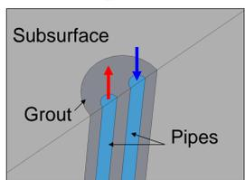
The model was validated with experimental data to assure that it works properly and represents the physical processes in a BHE. Since we are interested in oscillatory signals, we need to evaluate the solutions in terms of phase shift, frequency and amplitude. Therefore, **LiveLink™ for MATLAB®** is used to perform parametric studies and for post-processing the thermal response of the BHE system.
