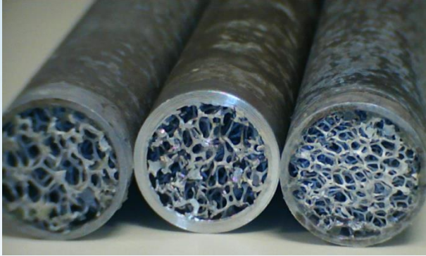
Test Objects: 3 types of aluminum foams brazed into 19mm(ID) x 200mm(L) tubes
