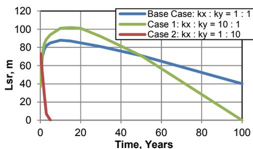
Figure 9. Analysis of anisotropic permeability
