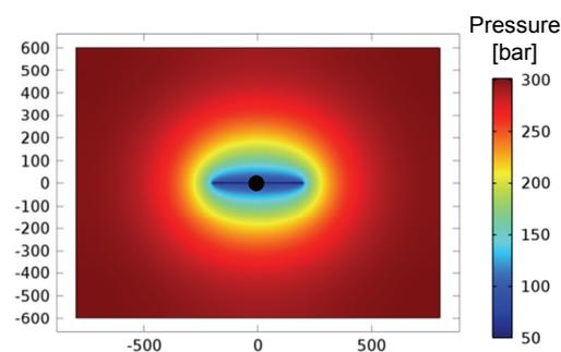
Figure 3. Fluid pressure distribution after five years
