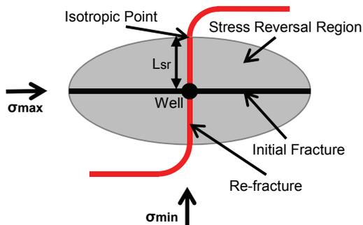
**Figure 1.** Schematic showing orthogonal fracture propagation (Redrawn after [6])
