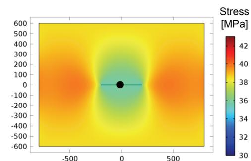
Figure 5. Stress tensor in y-direction
