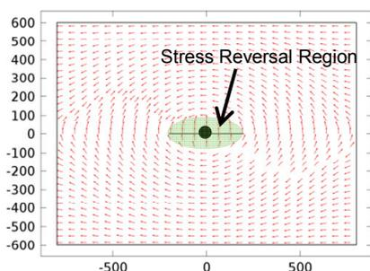
Figure 7. Maximum principle stress direction after five years
