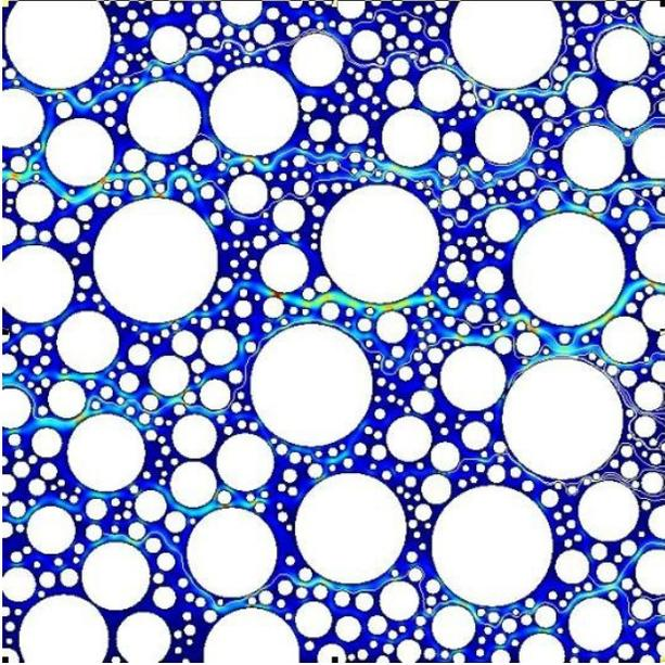
**Figure 1:** Laminar flow in a porous medium: velocity distribution.
