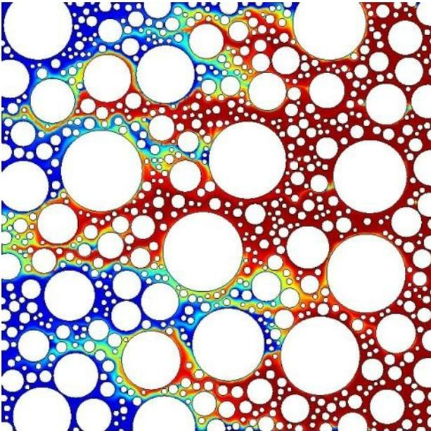
**Figure 2:** Tracer distribution in a porous medium.
