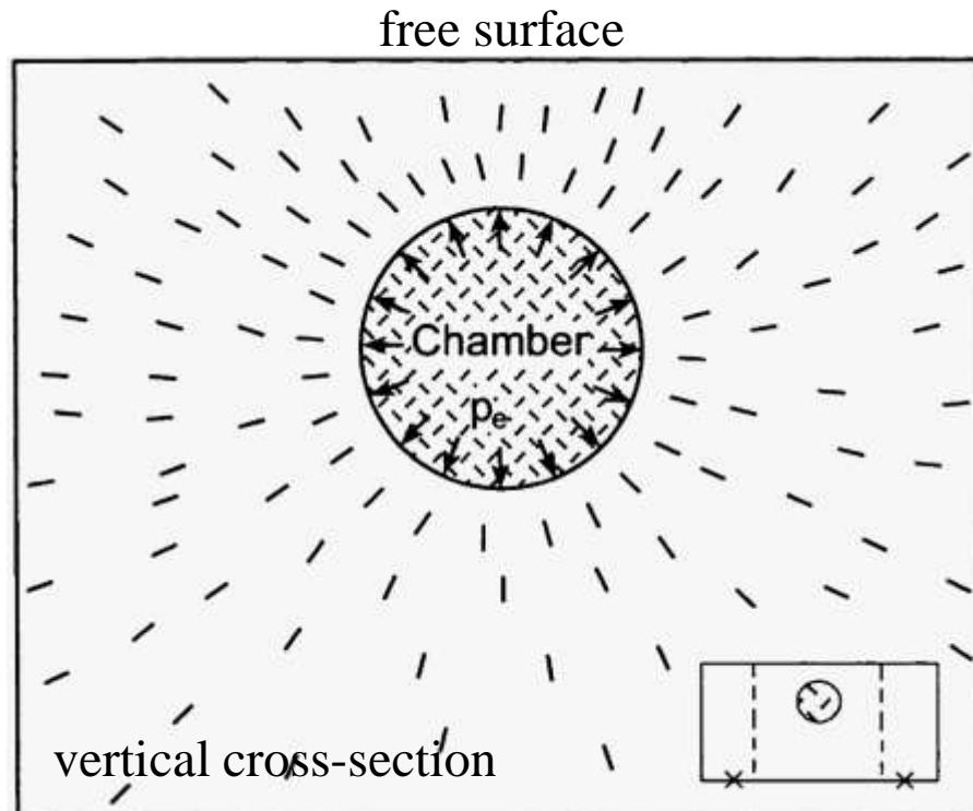
2D BEM or FEM model of a spherical magma chamber with overpressure.
