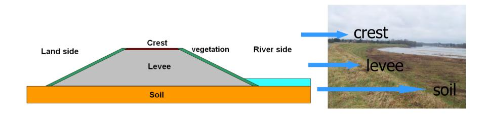
Typical cross-section of a levee alongside a river, like the Loire in France.
