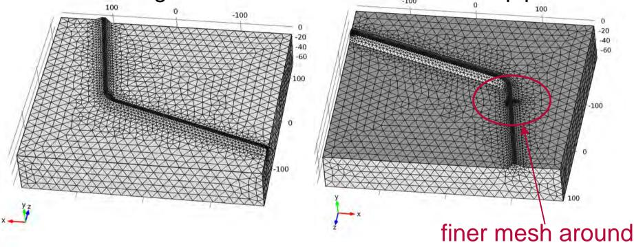
In the study: stationary and iterative solver the gas pipe with frequency domain,
