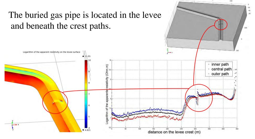
3D modelling of apparent resistivity amplitudes. This show the longitudinal profiles on the levee crest with a typical sinusoidal anomalie of a metallic pipe.
