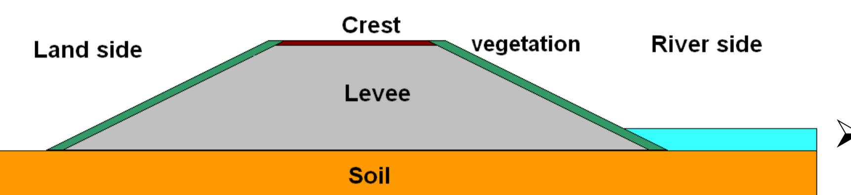
Typical cross-section of a levee on a river, like the Loire in France
