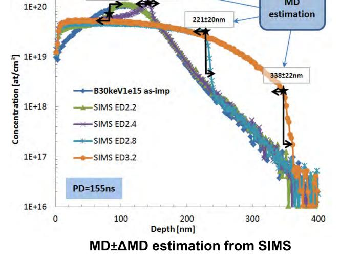
(profiles obtained by means of one pulse laser irradiation)
