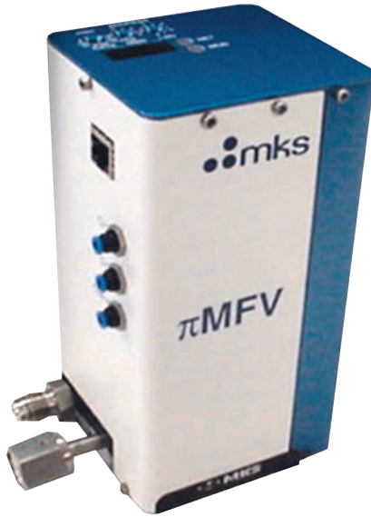
FIGURE 1: The \pi -MFV Mass-Flow Verifier measures the rate of change of pressure in a fixed volume. COMSOL Multiphysics helped the designers verify the accuracy of a condensed set of Navier-Stokes equations that run in real time on an embedded processor in the device.
