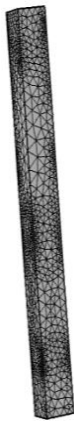
Figure 1. Rectangular cuboid light pipe (1mm 2 x10mm) with rough surfaces and ray simulation.
