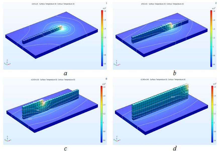
Figure 3. Kinetics of change of temperature fields in time: a – 20 s, b – 50 s, c – 100 s, d – 149 s.
