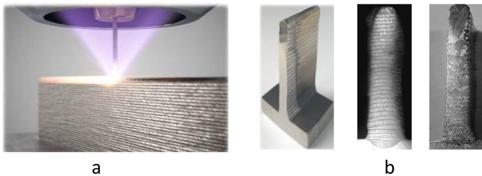
Figure 1. Electron beam surfacing (a) and structure of surfacing (b)
