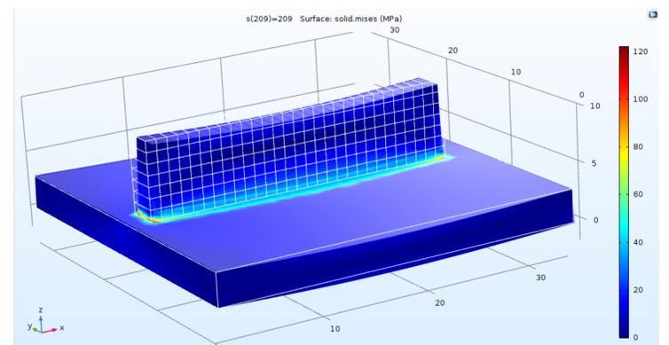
Figure 3. Stresses in deposition of 7 additive layers
