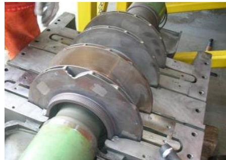
Figure 4 A typical failure of an impeller due to acoustic excitation.
