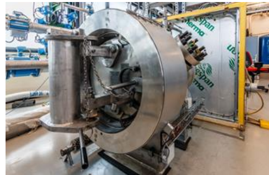
Figure 9 Test vessel with in the front the quick opening and closing door.
