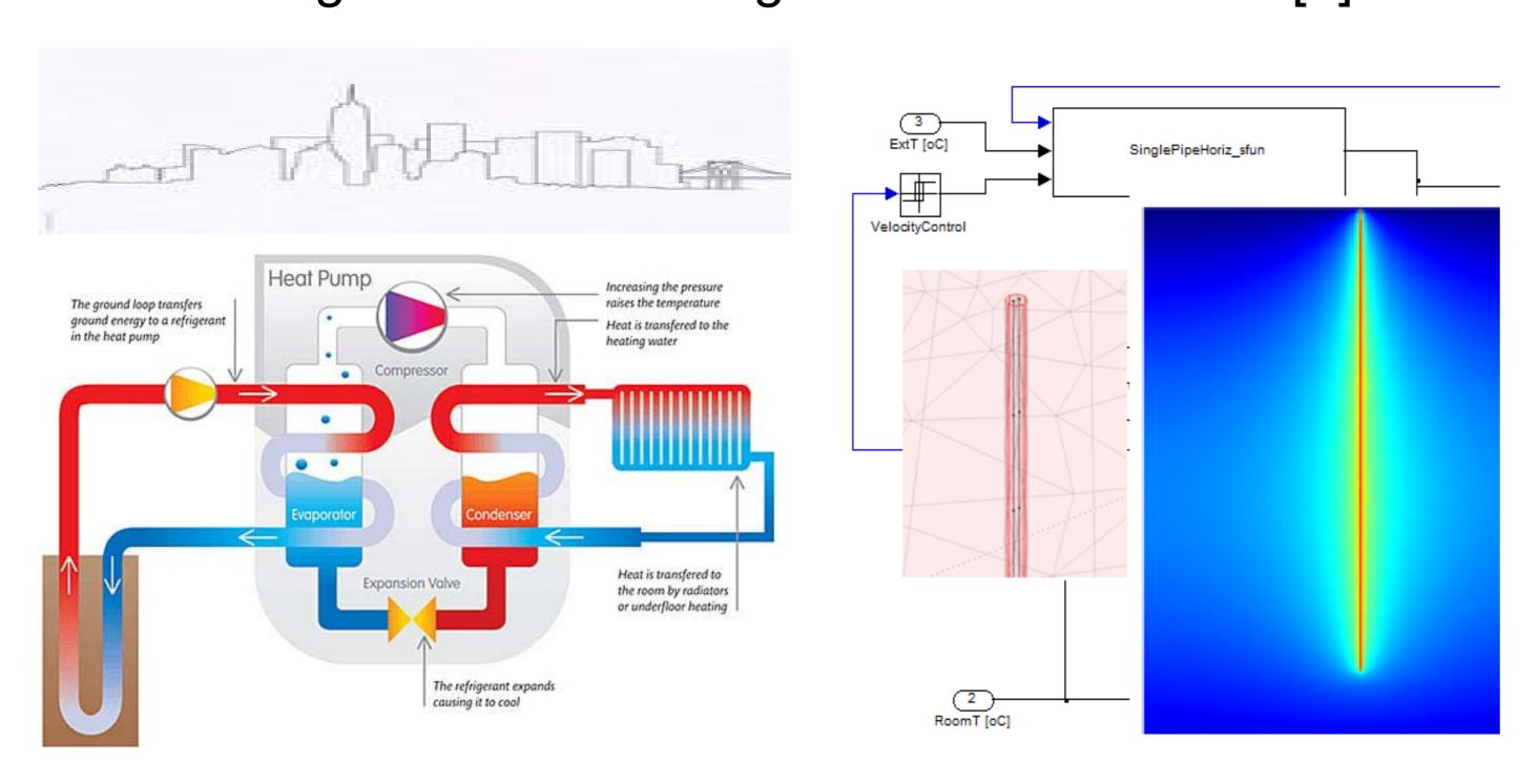
Impression of modeling: The heat pump and heat exchangers (Left) and the Comsol model of the bore hole integrated and controlled in SimuLink (Right)
