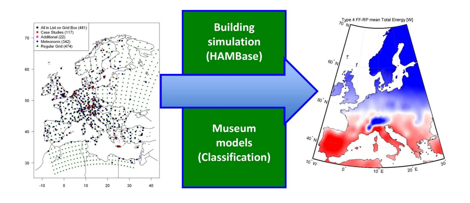
Impression of the methodology, using future external climate data form locations within the EU (Left) and simulated future indoor energy demand of a specific building for each location visualized in a map (Right).
