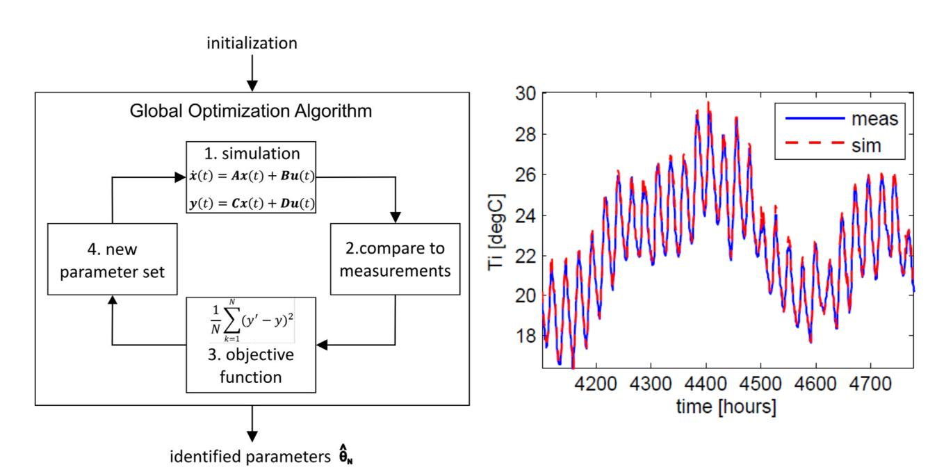
The methodology (Left) and the comparison of the measured and simulated temperatures of an indoor climate.
