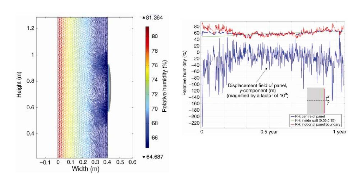
The relative humidity (RH) distribution of a wall and painting at a specific moment (Left). The displacement of the panel i.e. painting ,due to RH fluctuations.
