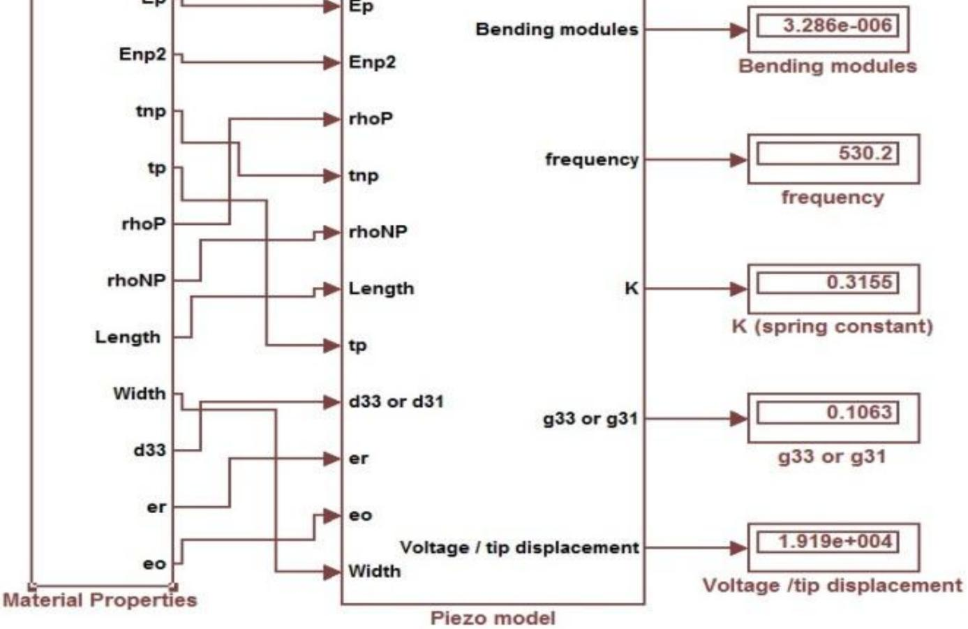
Fig. 1 Simulink model of piezoelectric unimorph cantilever
