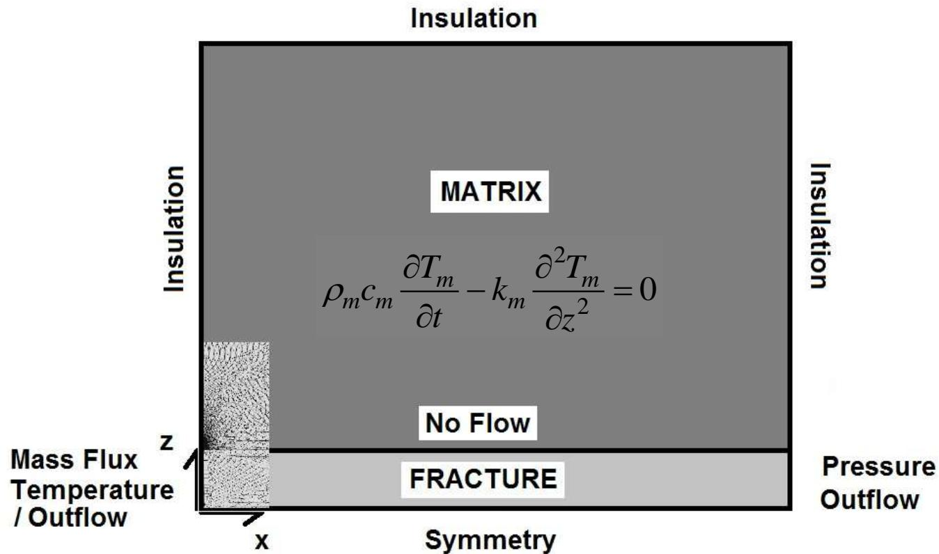
$$\left. \rho_f c_f \frac{\partial T}{\partial t} \pm \rho_w c_w \phi u \frac{\partial T}{\partial x} - \frac{k_m}{b} \frac{\partial T_m}{\partial z} \right|_{z=0} = 0$$
