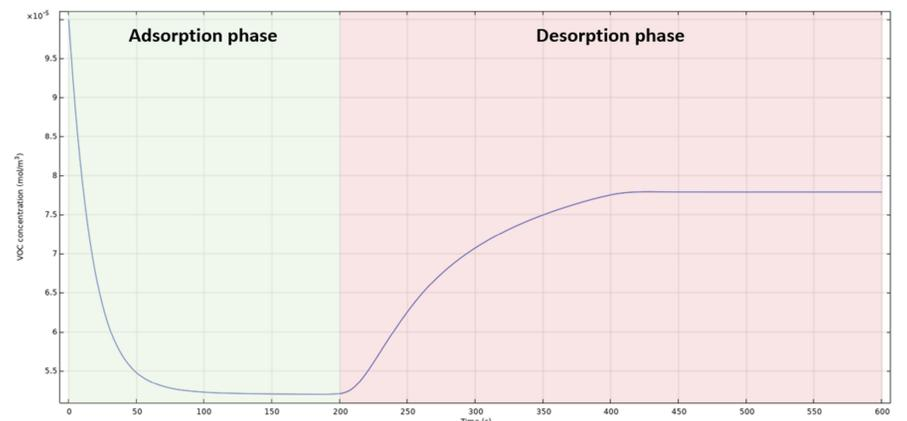
FIGURE 2. VOC concentration in reactor in adsorption and desorption phase.
