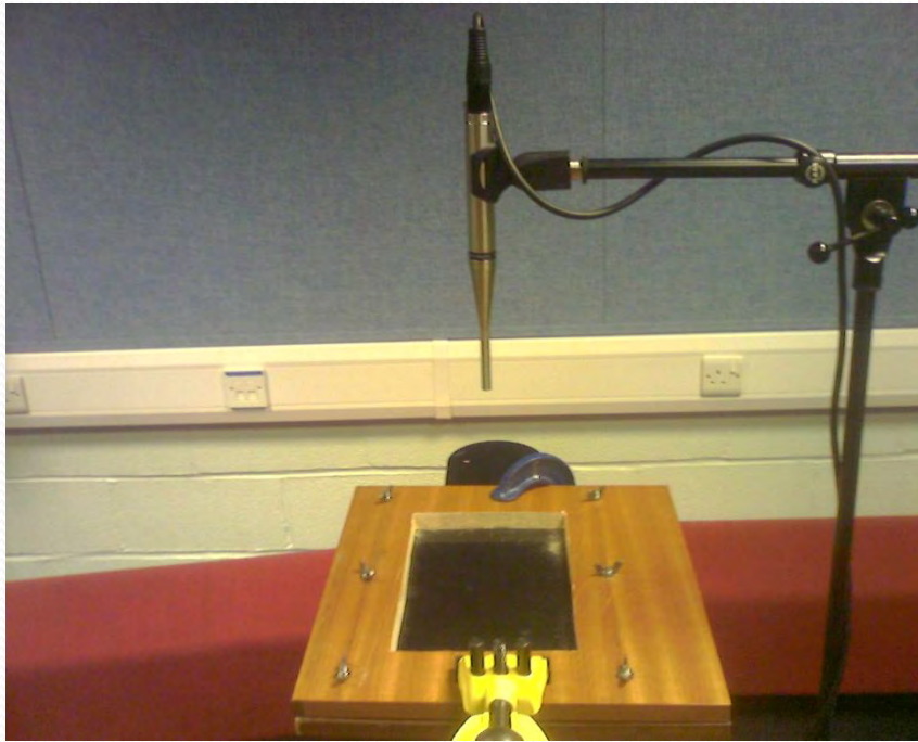
Figure 1 – Microphone position over clamped CFRP
